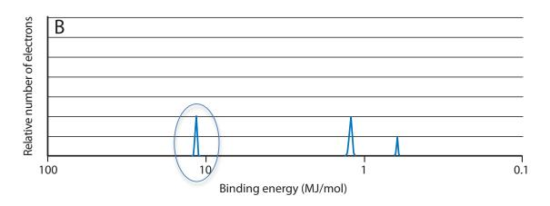
The electrons that would experience the greatest effective nuclear charge are the electrons that are closest to the nucleus, therefore the peak representing the 1s electrons at a binding energy of approximately 15 MJ/mol. These electrons are not affected by any shielding effect of other electrons therefore they are experiencing the greatest pull towards the nucleus.
